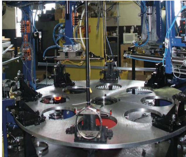
8 Stations Dial Assemble Machine with Vision Inspection Cameras
